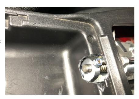
• Drill a hole about 15 mm in the front of the ashtray to ensure the clearance for the reverse gear locking pin.
