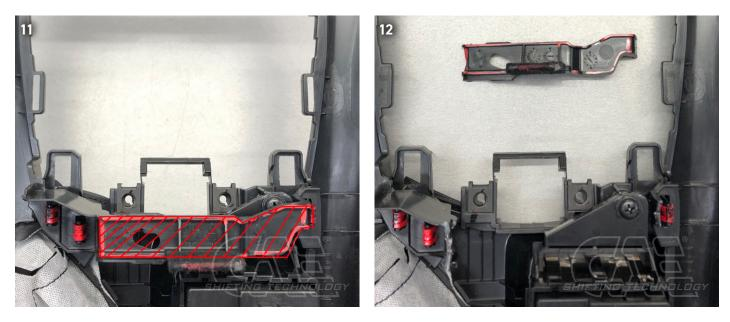
Mill out the switch unit of the center console in the area marked in red. (Picture 13, 14)
