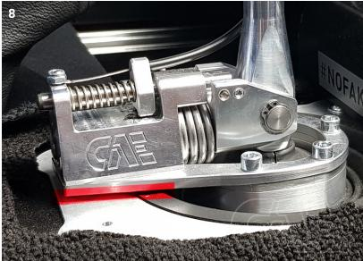
(i) Generally grease every bearing position regularly. We recommend Würth HHS 2000. Secure all nuts / screws with toothed lock washer or glue them in place during assembly!
