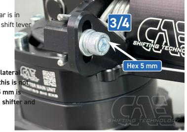
▶ Then shift the gearbox to level 1/2 using the shift lever and adjust the stop screw until the gears in level (1/2) can be changed cleanly. The adjusting screw should have a clearance of approx. 0.5 mm. (Picture 9)
