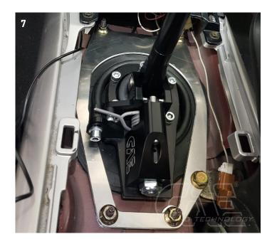
i PLEASE NOTE: There must be a gap of approx. 4-5 mm between the shifter and the transmission tunnel / collar plate. (Picture 7) If there is not enough clearance, loosen the 3 connecting screws of the PPF carrier on the gearbox and lift the gearbox slightly. Then tighten the screws again and check if there is enough space between shifter and gearbox tunnel.
