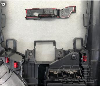
Mill out the switch unit of the center console in the area marked in red. (Picture 13, 14)
