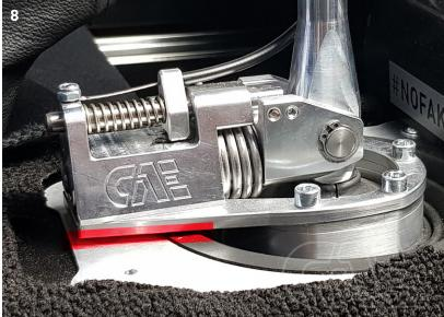
(i) Generally grease each bearing point of the shifter regularly. We recommend Würth HHS 2000. Secure or glue all nuts / screws with toothed lock washer during assembly!
