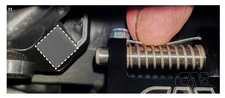
If desired, you can also reinstall the shift bag. To do this, the plastic frame in the area of the ashtray must be cut out and the bag at the upper end cut a little.
