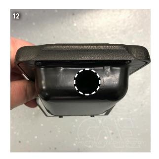
If desired, you can also reinstall the shift bag. For this you must cut out the plastic frame in the area oft he ashtray and the bag at the top. The original shift bag can be left or to be used.
