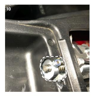
Drill a hole about 15 mm in the front of the ashtray to ensure the clearance for the reverse gear locking pin (Picture 11, 12)
