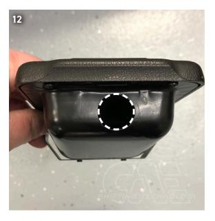
If desired, you can also reinstall the shift bag. For this you must cut out the plastic frame in the area oft he ashtray and the bag at the top. The original shift bag can be left or to be used.
