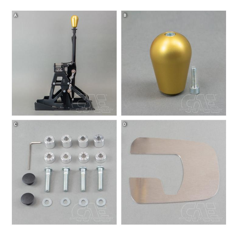
(i) The shifter is intended for vehicles with interior equipment. The center console must be trimmed slightly for installation until the appropriate clearance for the shifter is ensured. Lubricate all moving parts occasionally with good spray grease, e.g. by touching the rubber caps on the ball heads. For cleaning the aluminum parts we recommend commercial spirit.
