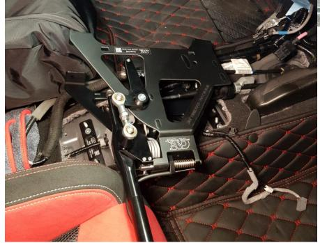
Position the CAE shifter and insert the shift cables into the shifter housing; Immediately insert the cables into the respective bracket and fasten by turning 90°. (cables do not lock)
