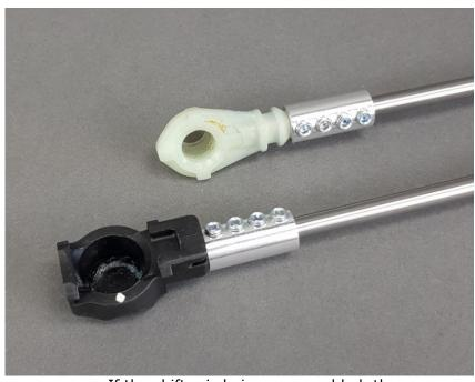
If the shifter is being reassembled, the supplied connection sleeves hast o be mounted as shown
