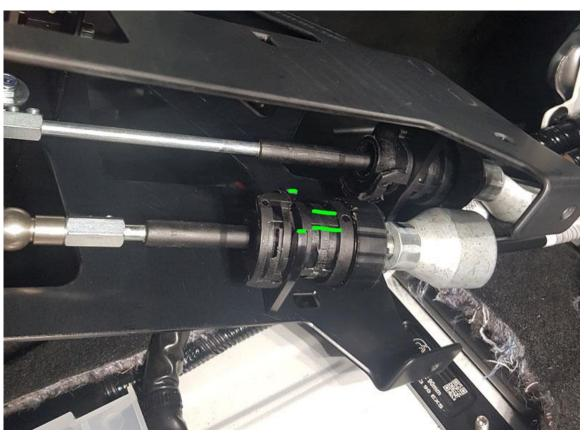
Then place the CAE Shifter on the bars and screw it tight with the 4 nuts.
