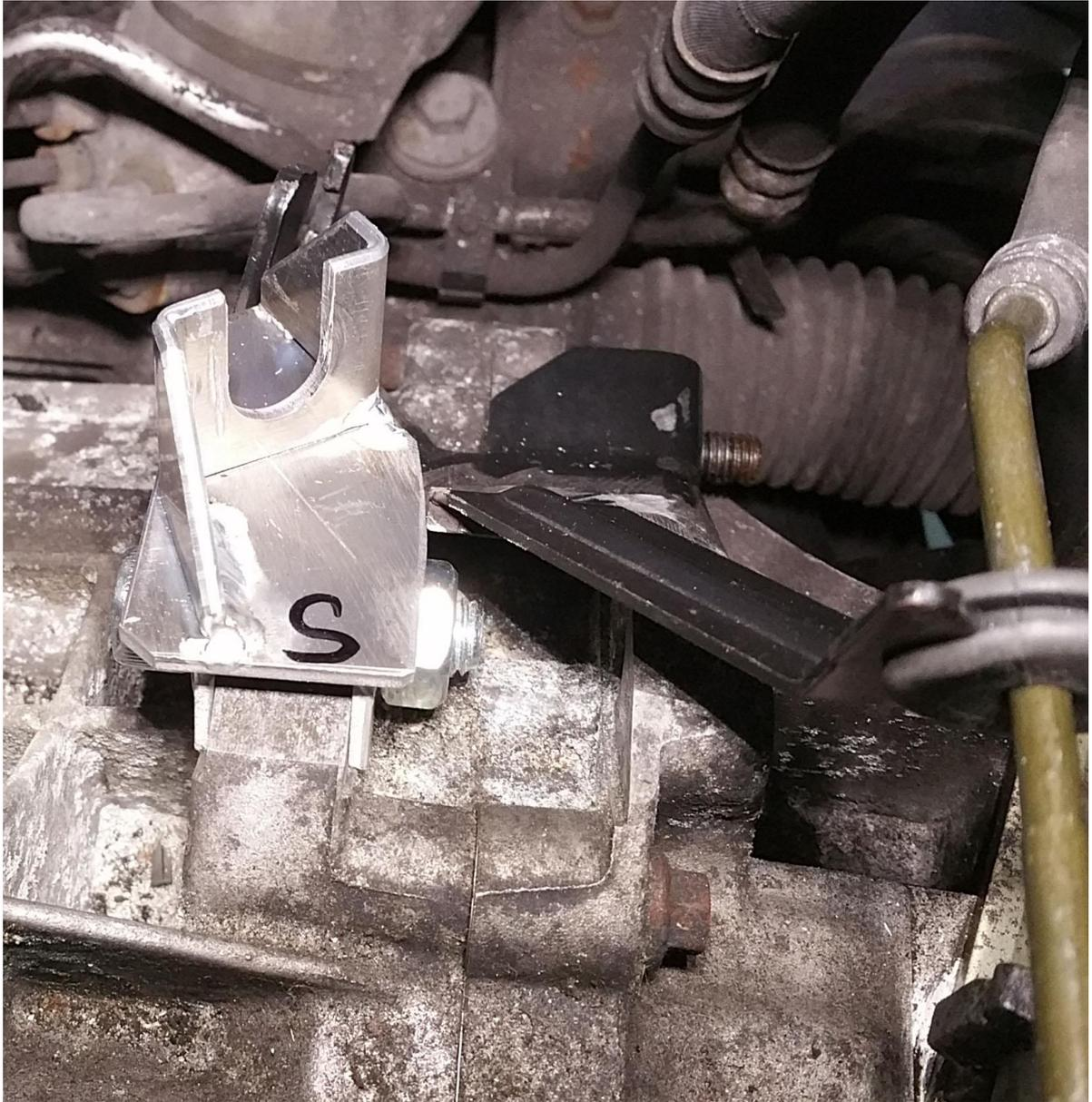
The original gear shifter must be removed from the stem:
