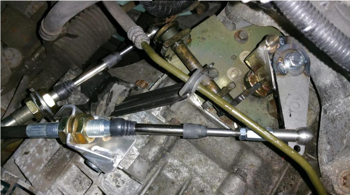
Mount the sealing collar on the selector lever ball head, grease the ball heads well
