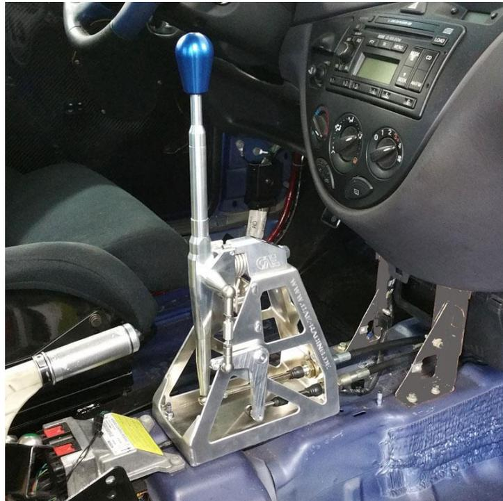
The shifter is intended for race cars without interior. When the center console is installed, it must be removed or cutted until a suitable clearance for the shifter is ensured. The shifter should be screwed directly onto the center tunnel, possibly existing carpet must be cut out.
