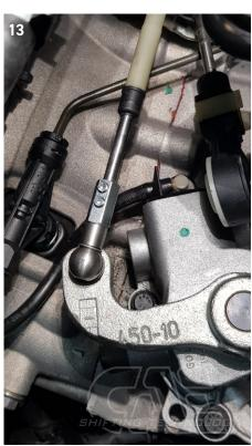
▶ Removal of the absorber weights on the gear lever also contributes to better shiftability; this is also recommended and not absolutely necessary for the function. (Picture 14, 15)
