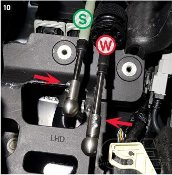
▶ We also recommend the conversion of the ball socket on the gearbox as this has a lot of clearance ex works to prevent vibrations from being transmitted. This is optional and not absolutely necessary for the pure function of the shifter. (Picture 11-13)
