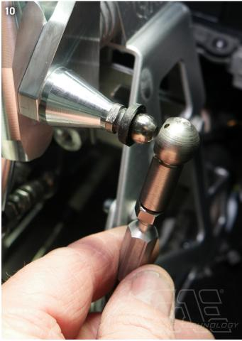
▶ Secure all ball cups of the coupling rods with the lock nuts.
