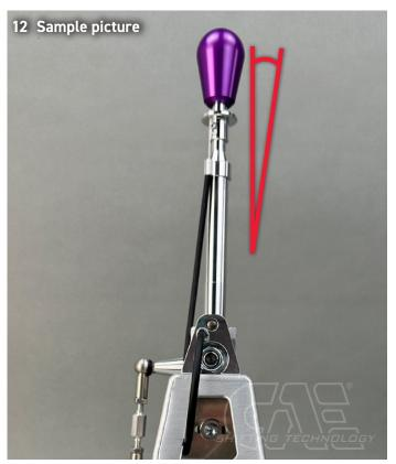
Secure all ball sockets of the coupling rods with the lock nuts.
