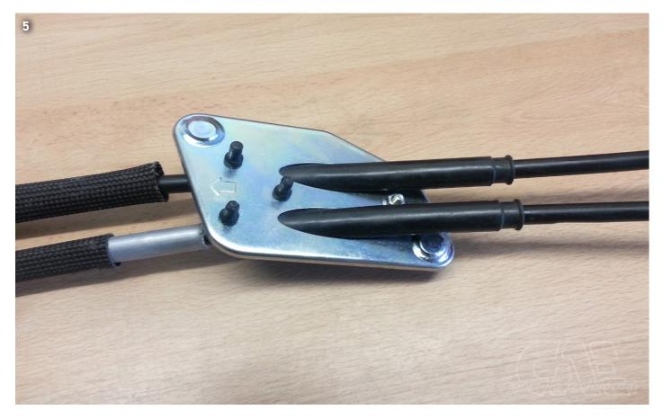
Bring the shifter with the shift cables already fitted to its installation location and move the shift cables through the bushing towards the engine compartment; screw the shifter onto the tunnel.
