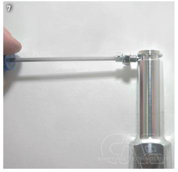
i Be sure to secure the grub screw at the end of assembly with the wire supplied.
