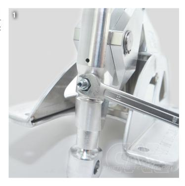
Mount the shift rod, after inserting the original 6mm bolt push the circlip out of the "parking position" into the notch.
