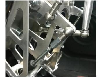
The standard metal ball pans of older vehicle models do not need to be rebuilt:
