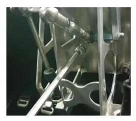
tighten the Shifter with 3 hex nuts and 1 inbus screw
