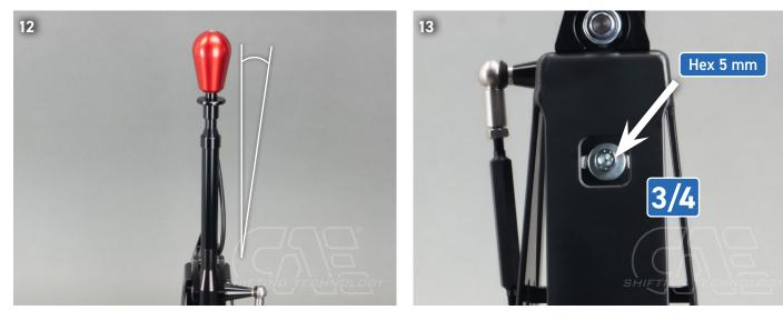
Shift the gearbox to 3rd or 4th gear by moving the shift lever forwards or backwards.
