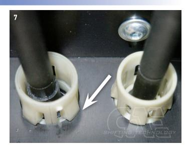
Secure the ball cups with the locking pins.
