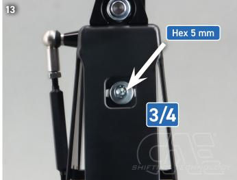
▶ Shift the gearbox to 3rd or 4th gear by moving the shift lever forwards or backwards.
