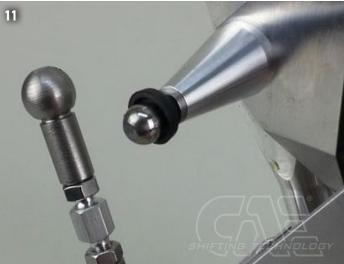
Find the center position of the shift lever. In the center position, the shift lever should be exactly vertical to slightly inclined (approx. 3 degrees) to the right. This can be adjusted under the gearshift bracket with a 5 mm Allen key by moving the lower spring stop. (Picture 12, 13)
