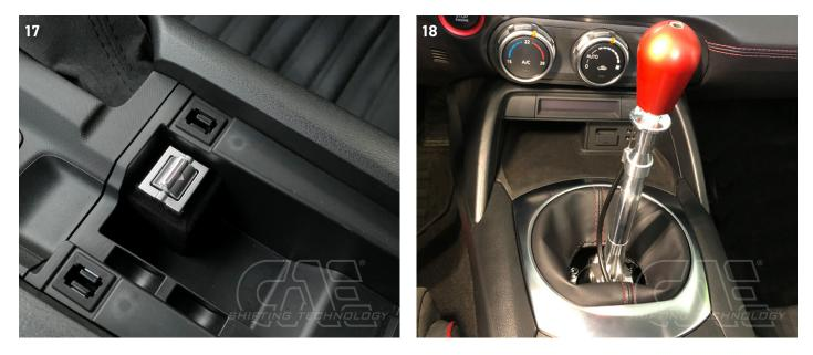
• The switch from the cover frame can be placed in the center console compartment.
