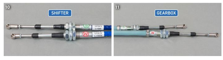
(i) PLEASE NOTE: ! Check cables for "end position free travel". When a gear is engaged, there must still be a residual travel available on the cable! (Picture A, B, C)
