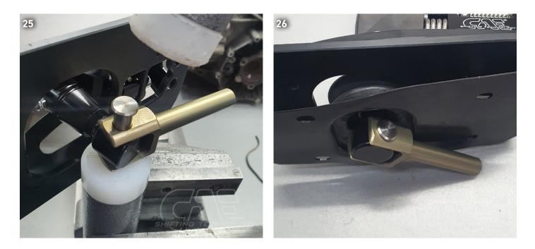
Mount the rubber bellows on the cover plate (please degrease first!) (Picture. 27, 28, 29). Mount the plate incl. rubber bellows on the shifter (as shown in Fig. 25). The upper bead of the rubber bellows must fit into the circumferential groove on the shifter. If necessary, use a few drops of brake cleaner as a lubricant.
