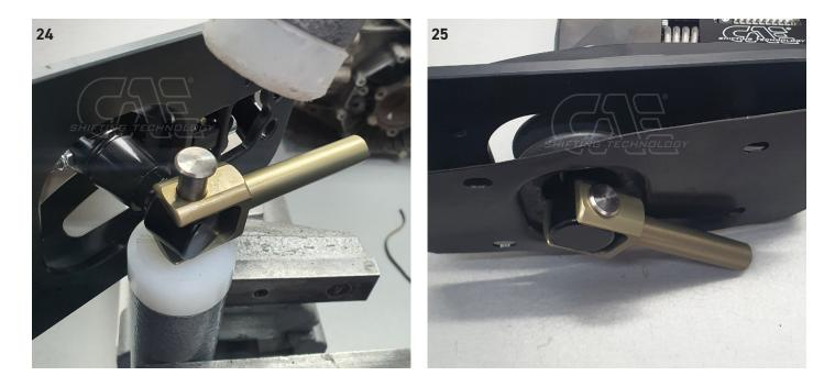
Mount the rubber bellows on the cover plate (please degrease!). Mount the sheet metal incl. rubber bellows on the shifter. The upper bead of the rubber bellows must be inserted into the circumferential groove at the shifter. If necessary, use a few drops of brake cleaner as lubricant.
