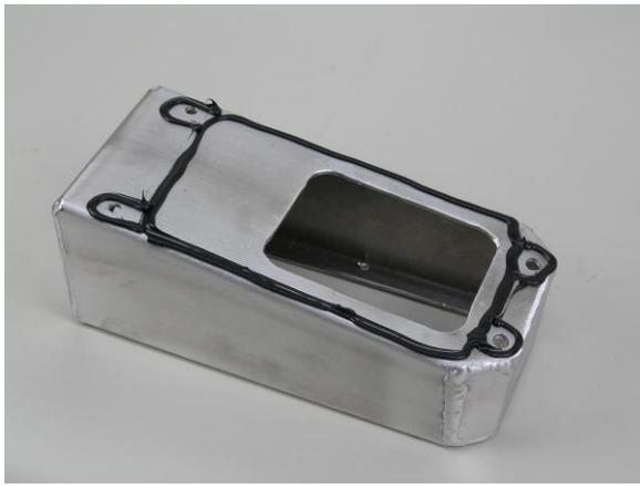
Mount the Box to the Tunnel from downside; use Hex screws M6x20. Use delivered self adheasing rubber stripe to seal it, or use body sealant
