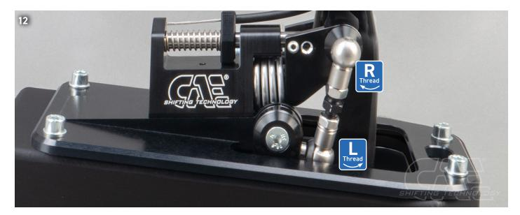
(i) PLEASE NOTE: ! Check cables for "end position free travel". When a gear is engaged, there must still be a residual travel available on the rope! (Picture A, B, C)
