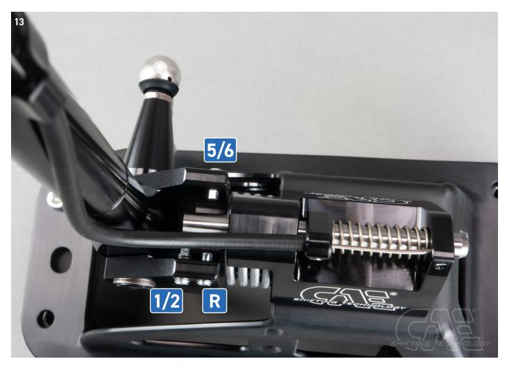
▶ Replace cover plate of shifter box with sealant and screw together, reinstall exhaust and cardan shaft. (Picture 14)
