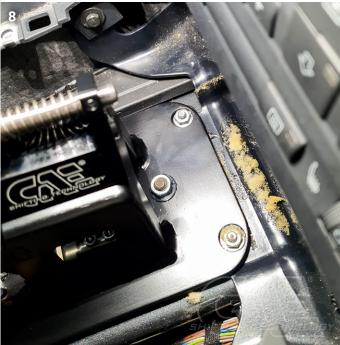
▶ Tighten the clamp only lightly at first; the exact setting is made in the next section. (Picture 9)
