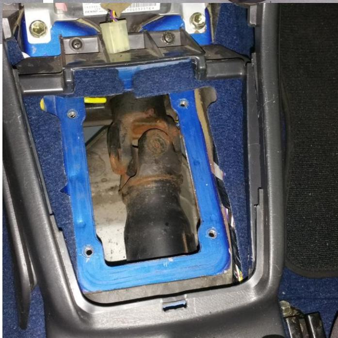
Disassemble the Shift unit to get the rubber boot as single part
