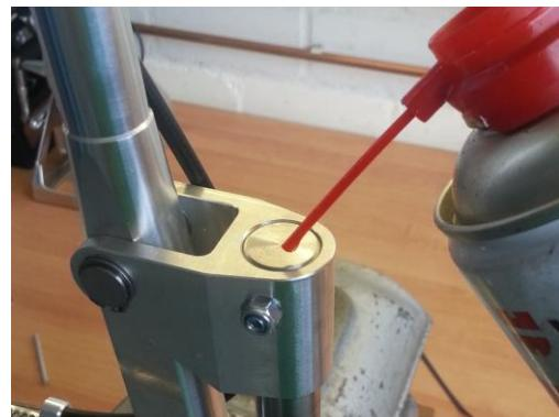
!!!Grease the Main bolt and the hole for it good before assambling !!!
